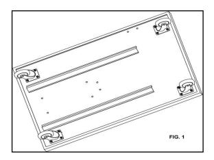
TO ASSEMBLY, FIRST PLACE THE BASE PLATE UPSIDE DOWN AND ATTACH THE FOUR CASTERS TO THE HOLES PROVIDED AND TOGHTEN WITH THE WRENCH. FIG.1
