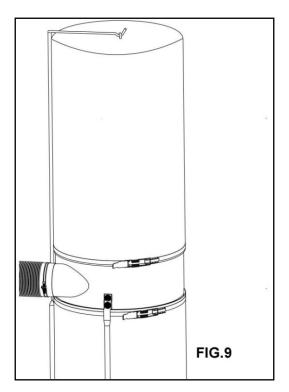
PLACE THE COLLECTOR AND FILTER BAGS ONTO THE COLLECTOR AND SECURE WITH THE BELTS AS SHOWN IN FIG.9.
