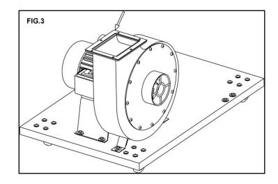
NEXT, MOUNT THE OUTLET , PACKING(I) TO THE COLLECTOR BODY AS SHOWN IN FIG.3 AND FIG. 4.
